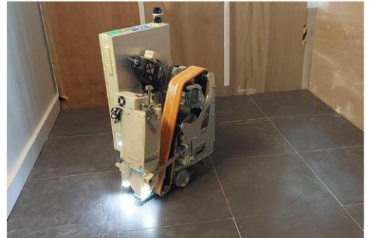
A robot by Singapore start-up Fabrica AI can apply grouting and clean tile gaps, and cover more than 90 per cent of unobstructed floor space. ST PHOTO: LEE YU HUI
